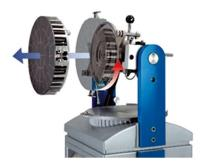
Interchangeable dividing disc (within 5 minutes) offers increased flexibility, a work range of 16 - 440 gr. and tilts forward for easy cleaning.
