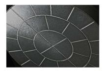
There's a choice of eight anodized coated aluminium dividing discs with stainless steel knives. The discs require minimal flour for dividing, are hygienic and can be cleaned in a dish-washer.
